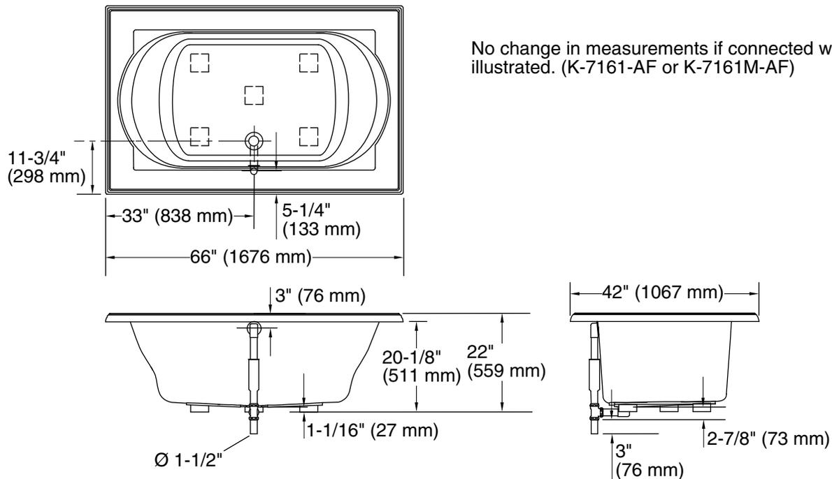
No change in measurements if connected with drain illustrated. (K-7161-AF or K-7161M-AF)
