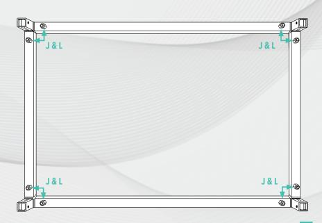
Align the Top Frame with the main frame and insert each Top Connector (C) into the appropriate Vertical Support (I).
