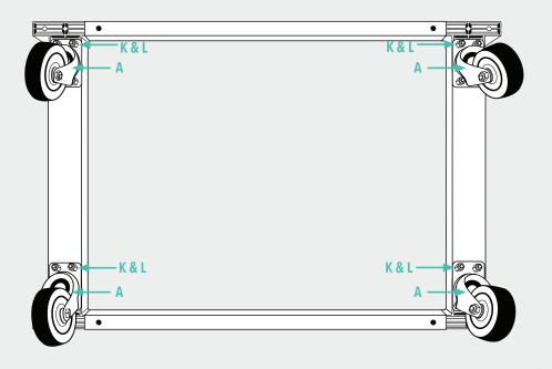
Insert four of the Frame Bolts (J) up through the Base Length Supports (E) securing with four Nuts (L). Use the appropriate tool to tighten.
