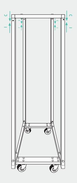
Secure the Top Frame to the Vertical Supports (I) by inserting a Frame Bolt (J) and Nut (L) through each.
