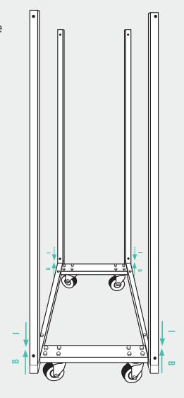
Insert four of the Frame Bolts (J) through the Vertical Supports and use a nut (L) on each to secure. Use the appropriate tool to tighten.
