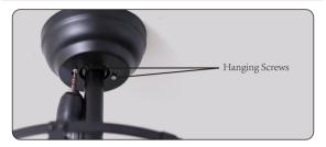
Align the cup notch with the screw on the bracket, lift the cup up and make the screws pass the cup notch, then screw in from the bottom up direction, and fix the four screws with the screwdrive, as shown in step 7.
