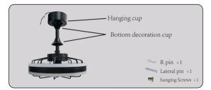
First pass the wires through the bottom decoration cup/hanging cup/hanging boom in sequence shown in Step 4.
