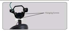
Place the hanging ball in the hanging bracket and turn the boom until the groove of the ball mesh with the lug of the plate.Please leave the two diagonal screws remained over half withdrew
