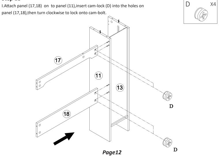
I.Attach panel (10) on to panel (17,18), insert cam-lock (D) into the holes on panel (17,18), then turn clockwise to lock onto cam-bolt.
