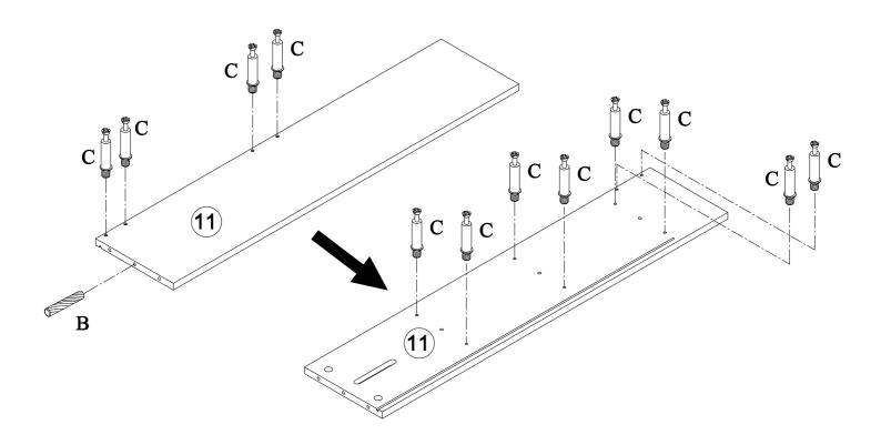
I.Screw in cam-bolt (C) into the designated holes on panel (10,12).
