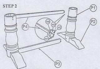
Assemble leg prongs P2 to both Pedestal Legs P1, then align Bottom Stretcher P3 and Top Rail P4 to connect both Pedestal Legs.
