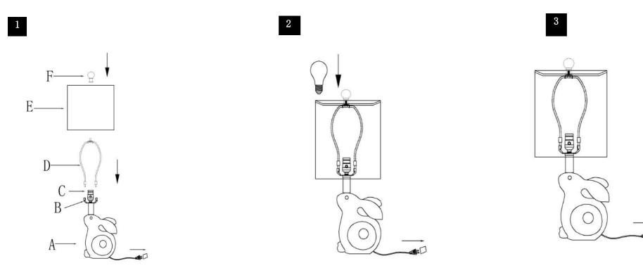
Step 1 Insert the Harp (D) into the Saddle (B). Put the shade(E) on the Harp(D), then tighten the Finial (F)into the Harp (D)
