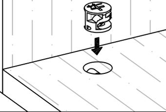
Screw the female camlock clockwise with a screwdriver.
