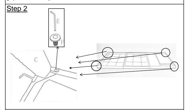
Attach Front&Back Leg((C) to the Seat Panel(A) using Bolt(F) with Allen Key(E).
