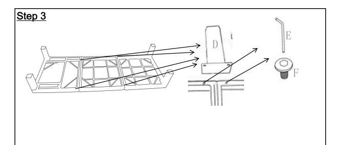
Attach Middle Leg((D) to the Seat Panel(A) using Bolt(F) with Allen Key(E).
