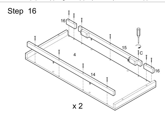
Attach slats (14,15,16) to leaf (4) using screws (C). Repeat this step for second leaf (4).
