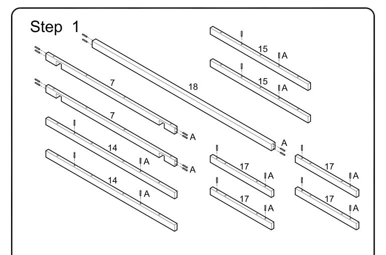
Insert dowels (A) into slats (7,14,15,17) and crossbar (18) as shown above.
