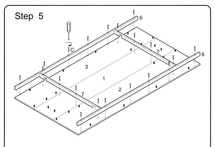
Attach slats (6,7) to table top pieces (1,2,3) using screws (C).
