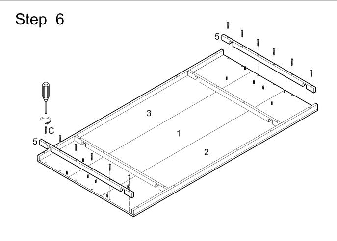
Attach slats (5) to table top pieces (1,2,3) using screws (C).
