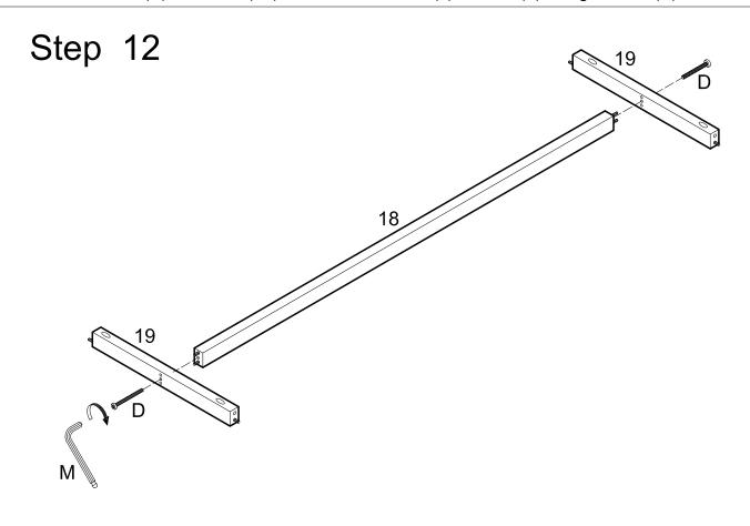
Attach crossbars (19) to crossbar (18) using bolts (D). Tighten bolts (D) with wrench (M).
