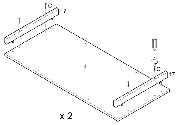
Attach slats (17) to leaf (4) using screws (C). Repeat this step for second leaf (4).
