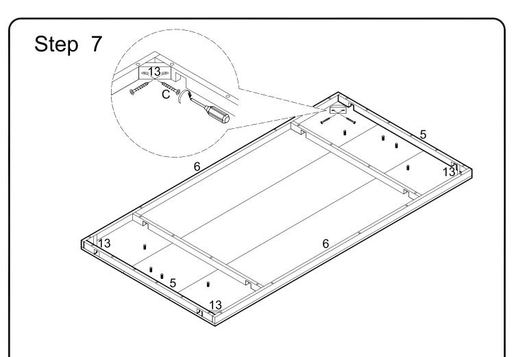
Attach corner blocks (13) to slats (5,6) using screws (C).
