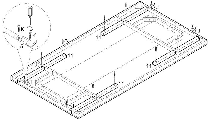
Insert dowels (A) into slats (11). Attach table locks (J) to slats (5) using screws (K).
