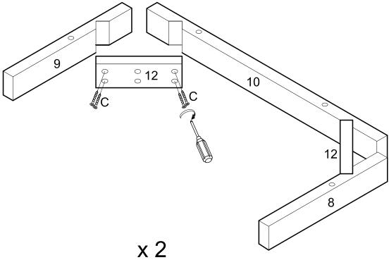
Attach corner blocks (12) to slats (8,9,10) using screws (C). Repeat this step for second set of slats (8,9,10).
