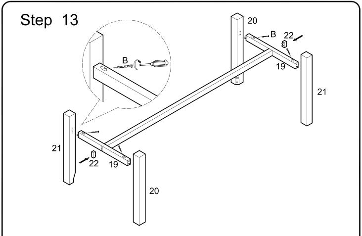
Attach crossbars (19) to legs (20,21) using screws (B). Attach end caps (22) to crossbars (19) using dowels as guides.
