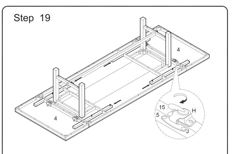
Pull slats (11) through leaves (4). Lock leaves (4) to main table assembly using table lock pieces (H,J).
