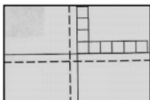
**Figure 2** Dry-lay a row of tiles from the center line to the side wall to determine the space left for the borders. If the resulting border is too small, move the starting point over a half tile width so that it straddles the center line. Repeat the same procedure lengthwise of the room. (This can readily be figured out from the room dimensions without putting down the tiles if desired.)
