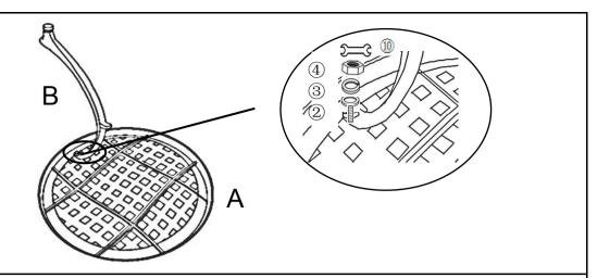
Attach the table leg with pre-attached Levellers(B) to the table top(A) using washers(②),spring washers(③),and nuts(④) with spanner(⑩). **DO NOT OVERTIGHTEN**.
