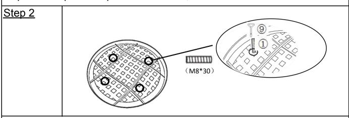
Lay the Table Top(A), facedown, onto a flat, soft, clean surface and lock the mounting positions with bolts(1) by using Screwdriver(9).
