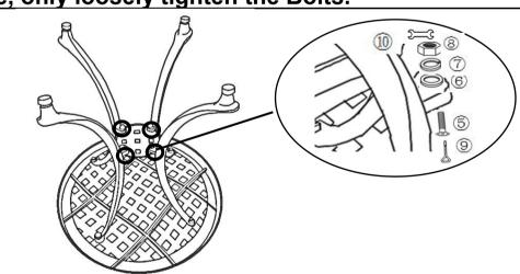
Loosely attach the round support (C) to Table Leg with pre-attached Levellers(B) with nuts(\$), washers(7), spring washers(\$) and bolts(\$), using the spanner(\$).
