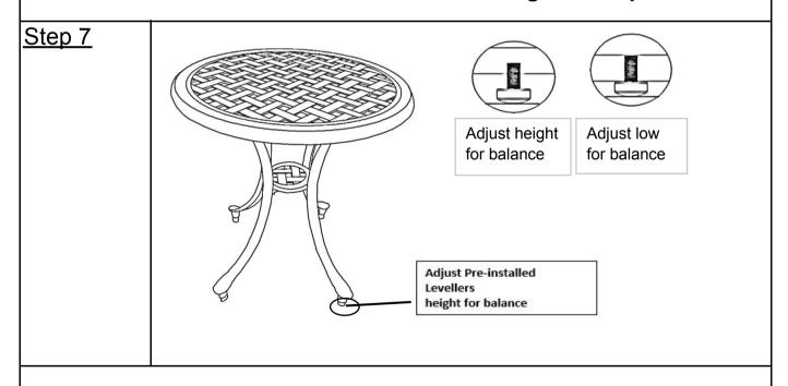
Adjust the Legs pre-installed Levellers until the Table is level with the ground.
