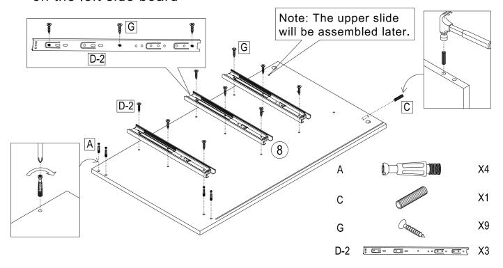
4. Assemble the slides, cam lock and wooden dowel on the right side board
