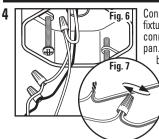
Connect the supply leads from the electrical box to the fixture wire leads using the wire nuts (**Fig. 6**). The connections need to be made on the back side of the pan. The black lead from the fixture pan is spliced to the black supply lead, and the white lead from the fixture pan is spliced to the white supply lead. Ensure the wire nuts are tight (**Fig. 7**). Carefully push the spliced wires back into the electrical box.
