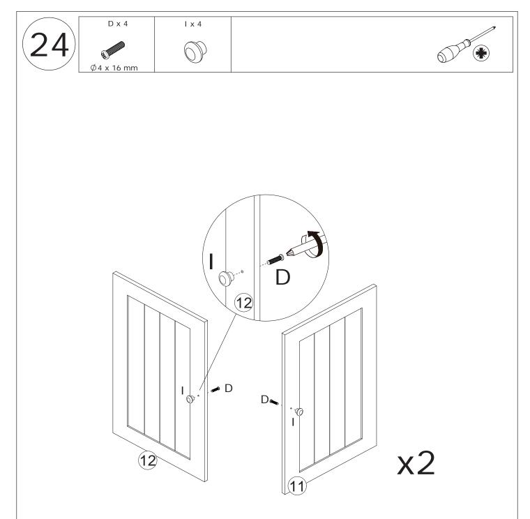
Fix knob(I) to plate 11 and 12 using screw(D) as shown.
