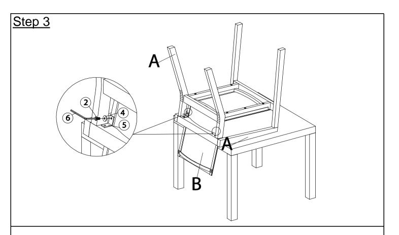
Attach L-Bracket(5) to Seat Frame(B) using Bolts(2) and Washers(4) with Allen Key(6).
