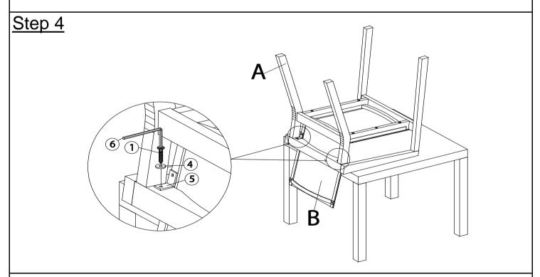
Attach L-Bracket(5) to Chair Frame(A) using Screws(1) and Washers(4) with Allen Key(6).
