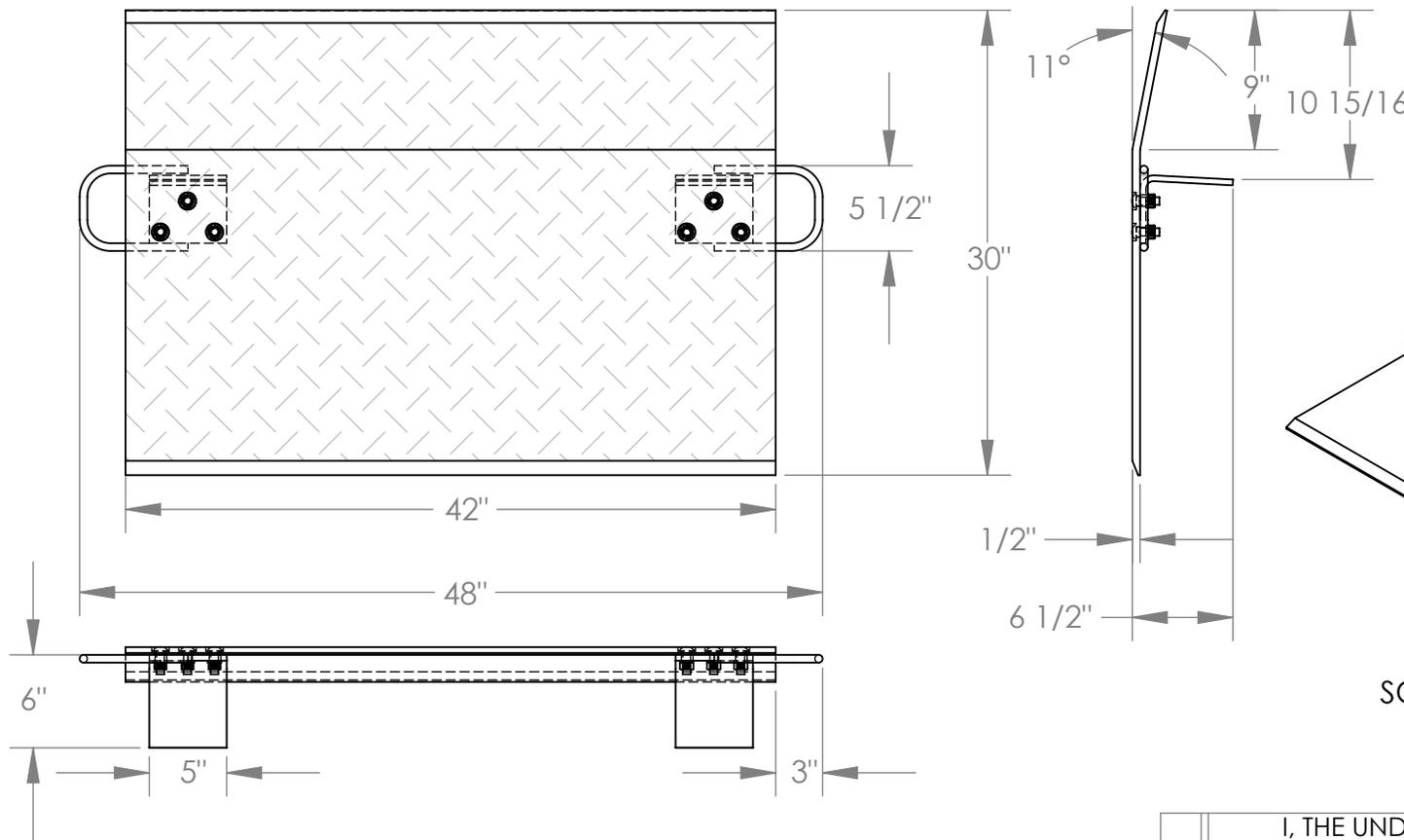
NOTE: BEND OR CROWN IS 11° AND LOCATED 9" FROM EDGE OF DOCKPLATE
