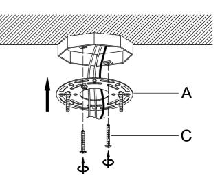
**Step 4:** Fix the Mounting Plate(A) to the junction box with Mounting Screw (C).
