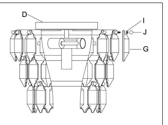
**Step 2**:Place the hole of the Crystal (G) on the exposed thread of the Lamp Body (D) .Then put on the Rubber Pad(I). rotate the Ball Nut (J) clockwise to hold it in place. Repeat this action. Load from the bottom to the top until all the crystals are covered.
