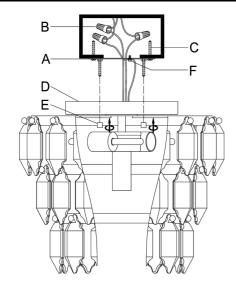
**Step 5:** Attach the Lamp Body(D) to the junction box and fix it by turning the Canopy Nut(E) clockwise.
