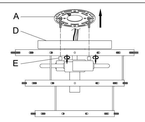
**Step 1**: Unpack all parts from cartons carefully.Turn the Canopy Nut (E) counterclockwise to separate the Mounting Plate (A) and Lamp Body (D).
