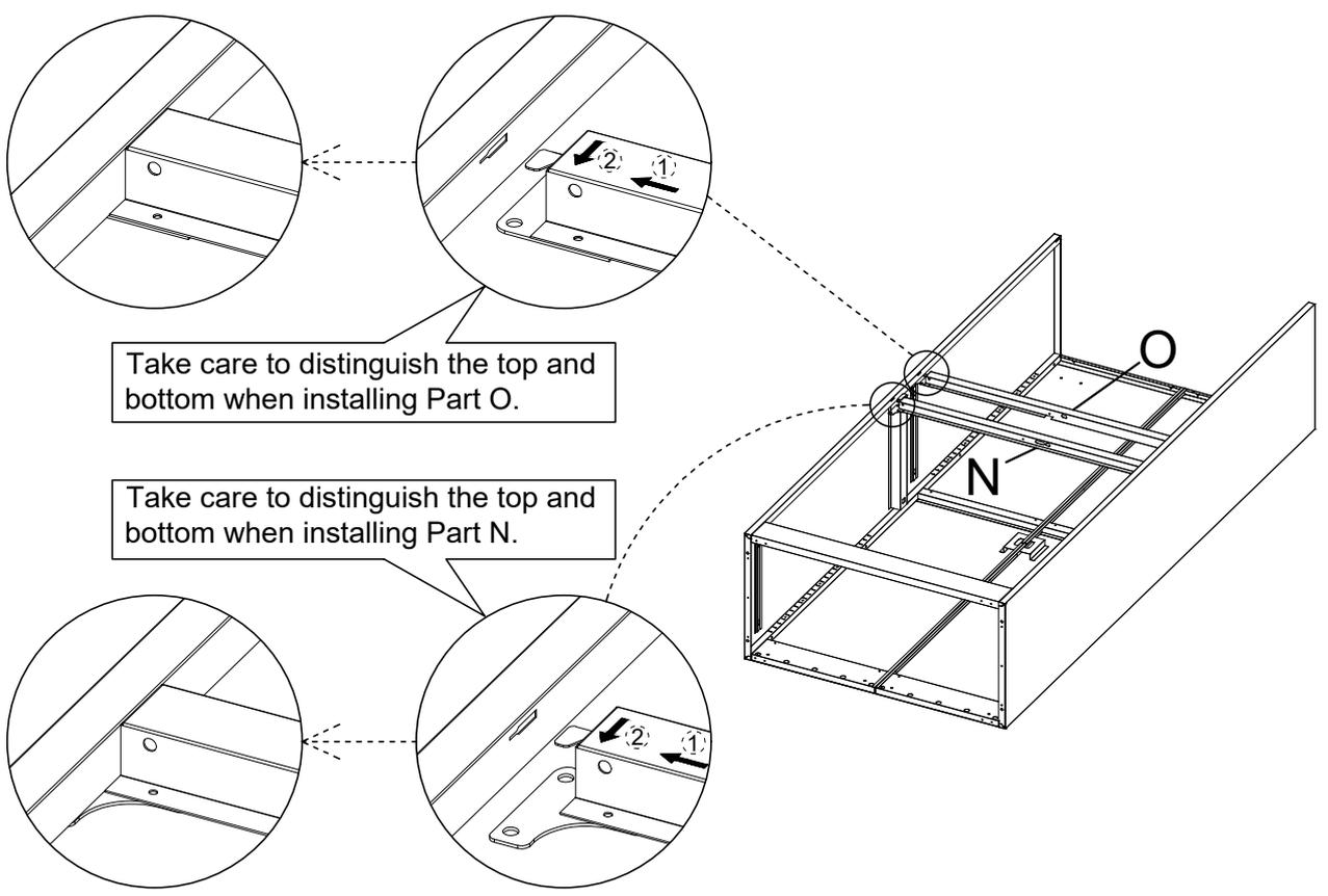
Take care to distinguish the top and bottom when installing Part O.
