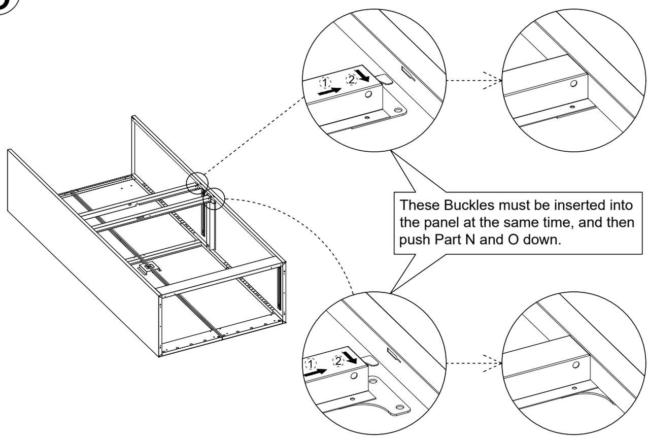
These Buckles must be inserted into the panel at the same time, and then push Part N and O down.
