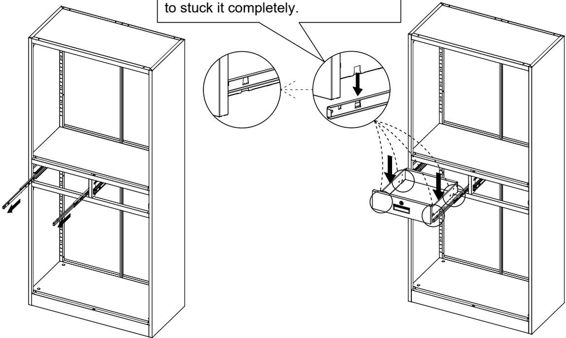
Pull out the two Guide Rails completely at the arrow position.
