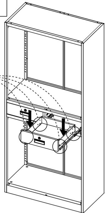
Pull out the two Guide Rails completely at the arrow position.
