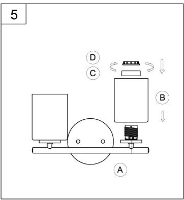
Screw lamp (not included) into fixture socket.
