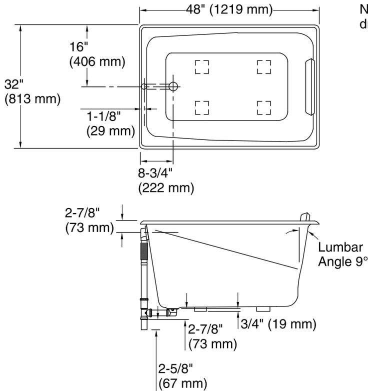
No change in measurement if connected with drain illustrated. (K-7265)
