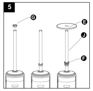
6. Insert the screw coupler (D) on the post (J), inserting it through the middle of the table (E) on the post (J). Thread the tightening spacer (F) on the bottom of the table (E) counterclockwise onto the screw coupler (D). Tighten securely to hold the table (E) to the screw coupler (D). Thread the fastening nut (G) counterclockwise. Tighten securely to lock in place. Loosen the fastening nut (G) to adjust the position of the table (E) on the post (J).
