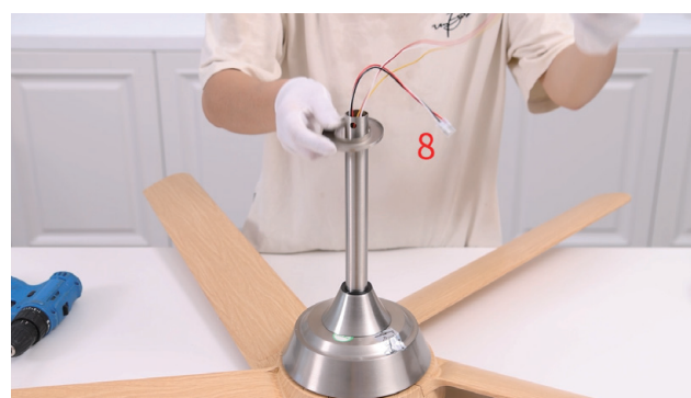
21. Put the hanger ball through the downrod
