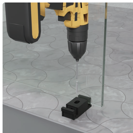
5/ Fix the glass guide block with screw
