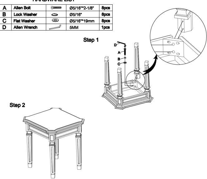
\*\*Note:Do not tighten all the bolts and the screws until the table has been put on a flat surface to adjust & level all the legs so that they do not wobble .Once adjusted then tighten all the bolts and the screws but not over-tight the bolts and the screws .
