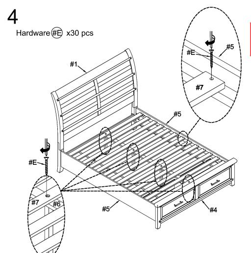
Align slats (#7) onto slat (#6) and side rails (#5), then secure by using screws (#E).
