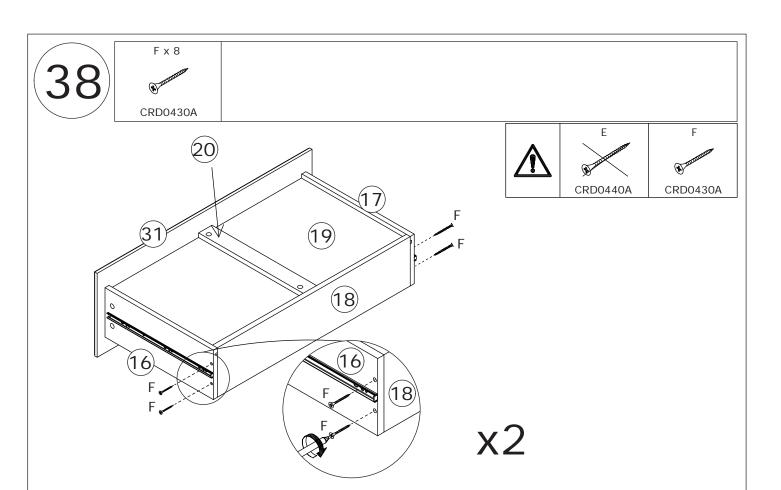
Fix plate 18 to plate 16 and 17 with screw(F) as shown.
