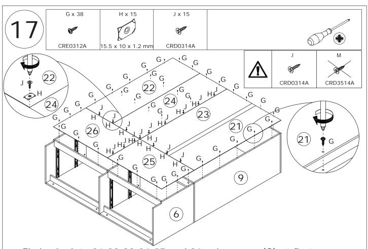
Fix back plate 21,22,23,24,25 and 26 using screw(G) at first. Fix each plate together using iron sheet(H) with screw(J) as shown.
