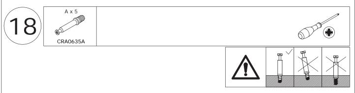
Insert quickfit screw(A) into plate 32 as shown.
