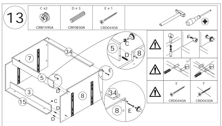
Attach plate 3, 15 and 5 to plate 8 with wooden dowel(D) at first. Put cam lock(C) into holes in plate 3,5 and turn clockwise to tighten as shown. Fix plate 8 to plate 34 with screw(E) as shown.
