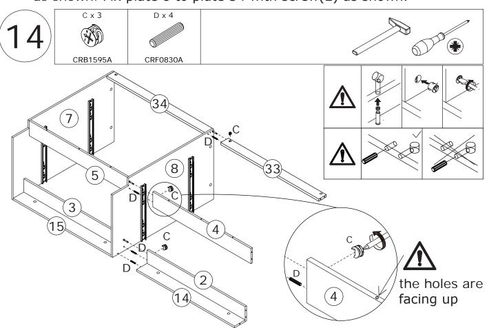
Attach plate 2,14,4 and 33 to plate 8 with wooden dowel(D) at first. Put cam lock(C) into holes in plate 2,4,33 and turn clockwise to tighten as shown.
