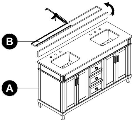
9.2 Removing silicon to the backsplash. Gently remove excess glue from the connecting area.
