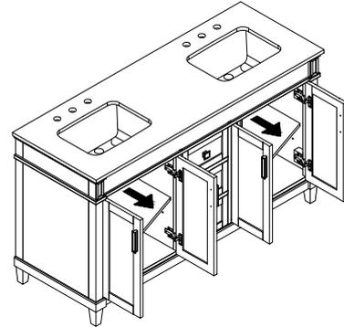
8.3 Inserting the shelf supports into the desired holes. Ensure that all the shelf supports are level.
