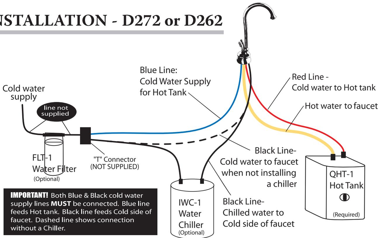
**IMPORTANT!** Both Blue & Black cold water supply lines **MUST** be connected. Blue line feeds Hot tank. Black line feeds Cold side of faucet. Dashed line shows connection without a Chiller.
