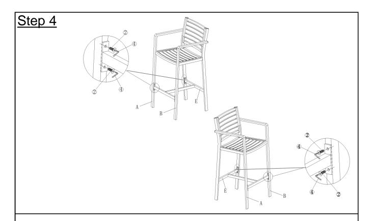
Attach Footrest(E) between Right Leg(B) and Left Leg(A) using Bolts(②) with Allen Key(④) as shown above.
