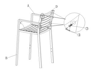
Attach Backrest(D) between Right Leg(B) and Left Leg(A) using Bolts(③) with Allen Key(④) as shown above.
