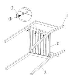
Attach Right Leg(B) to Seat(C) using Bolts(1) with Allen Key(4) as shown above. **Do not fully tighten the Bolts.**
