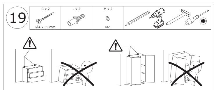
Once assembled lift furniture into place, do not drag. Use a drill to create a small hole lining up with the top of the safety strap (M3). Fasten to wall using wall anchor (L), washer (M2), wall screw(C). Ensure the unit is balaced and steady before use. You're done, enjoy
