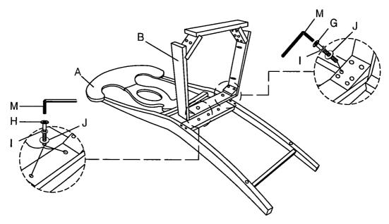
Take the Allen Key, and turn the bolts until the legs are secure. DO NOT TIGHTEN COMPLETELY.
