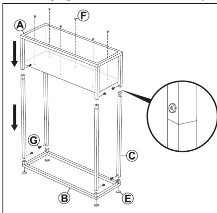
Apply four Protective Feet (E) to the bottom of Base (B).
