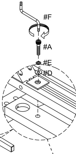
2. Prepare 2 bolt assemblies by first inserting a lock washer (#E) onto the bolt (#A) then a flat washer (#D) onto that same bolt (#A). Then insert the bolt assemblies into the holes along the seat panel (#2) and secure using the Allen wrench (#F).
