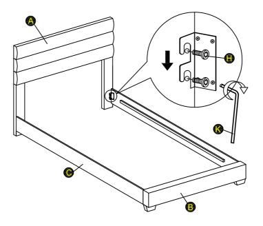
Attach the complete Side Rails (Part C) to the Headboard (Part A) and Footboard (Part B) with eight 20mm Bolts (Part H) to the headboard leg and footboard using the Small Hex Key (Part K). Do not tighten.
