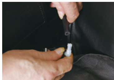
Connect air tube of armrest.
