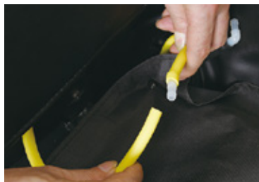
Connect air tube of near seat.
