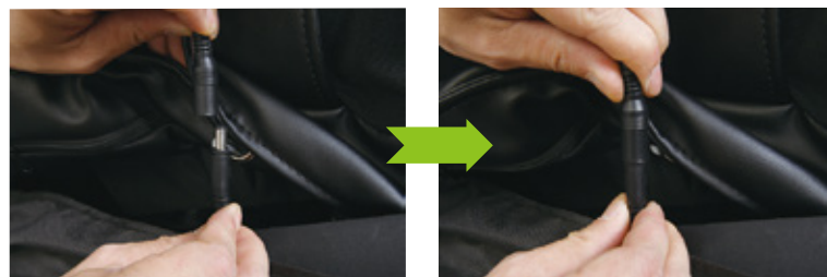
Connect back cushion heat wire.
