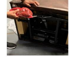
The transformer for a lift chair has two cables, one that goes from the wall plug to the transformer, and one that goes from the transformer to the chair.
