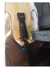
Picture shows a properly aligned KD bracket.
