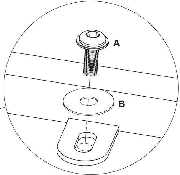
2. Turn it over and put it right. Adjust 4 legs land on floor , then tighten the screws slowly. During this process, please tighten screws while adjust legs balance until all the screws are tighten enough.
