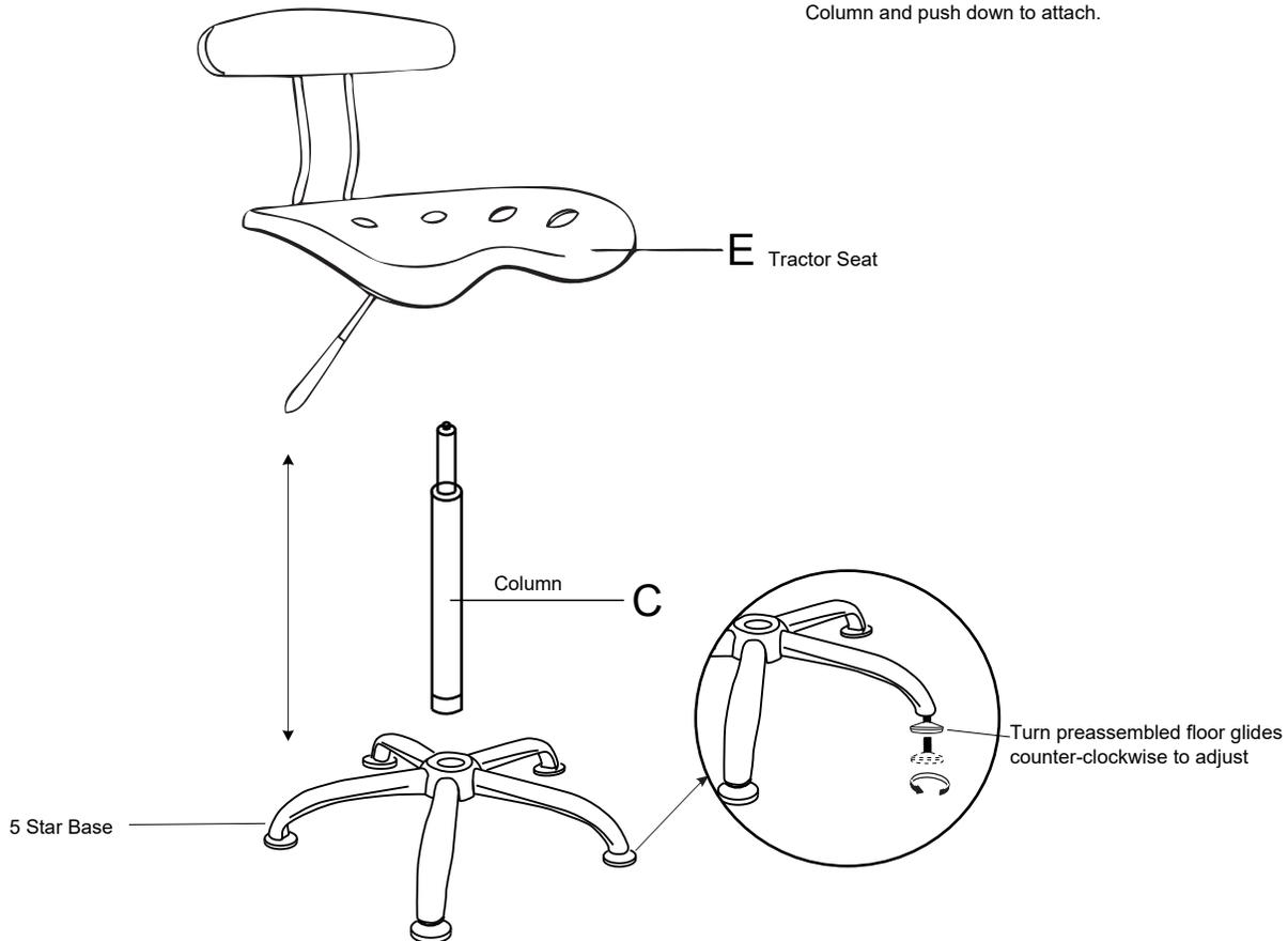
**STEP 4:** Insert larger end of the Column (Part C) into the 5 Star Base (Part A). Place the assembled seat onto the Column and push down to attach.
