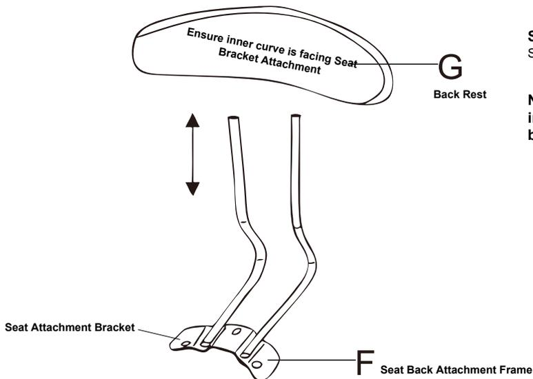
**STEP 2:** Push Seat Back (Part G) onto posts of Seat Back Attachment Frame (Part F).
