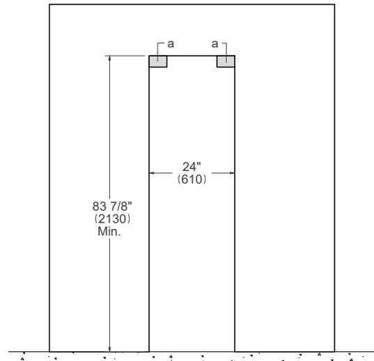
(a) Area to be left clear for the anti-tipping brackets – 3 1/2x5" (82x127mm)
