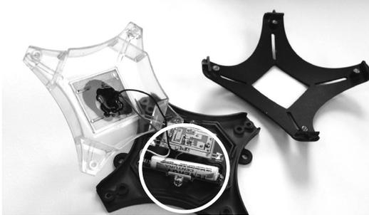
5. Once the battery is replaced, replace the clear plastic lens cover and outer metal cover and secure by replacing the screws removed in steps 1 and 2.
