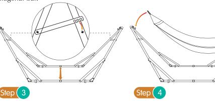
Expand the hammock base stand vertically. Connect the cross bar to the notch on the opposite main bar.
