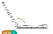
Put the base stand horizontally on your chosen surface. Extend the main diagonal bar.
