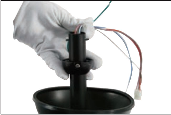
Step 7 Fix the motor to the hanging bracket.
