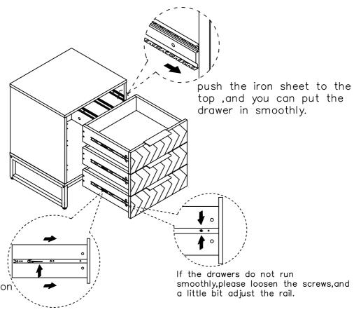
press down the device on the guide so that the drawer can be removed from the filing cabinet.
