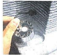
Find the groove on the product with a wire hole nearby, as shown in the figure.
