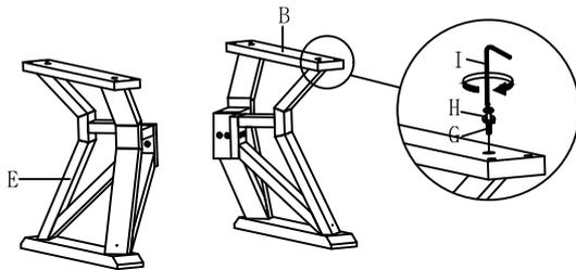
**Step 3:** Attach Table Leg E with Center Support D by insert (I, H & F).
