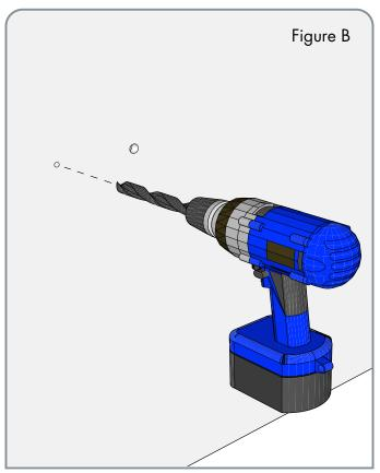
**2a. Drill anchor holes for drywall –** Drill 1/16 in pilot holes to determine if the holes are over a stud. Drill ½ in (13.7mm) hole for the Toggle Bolts centered on the marked hole locations.
