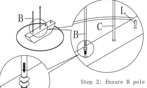
Step 2: Ensure B pole is rotated to the groove.
