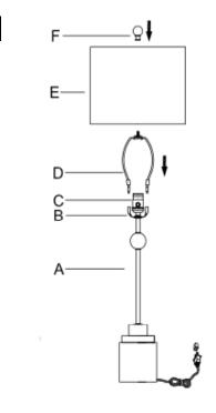
Step 1 Insert the Harp (D) into the Saddle (B). Put the shade(E) on the Harp(D), then tighten the Finial (F)into the Harp (D)
