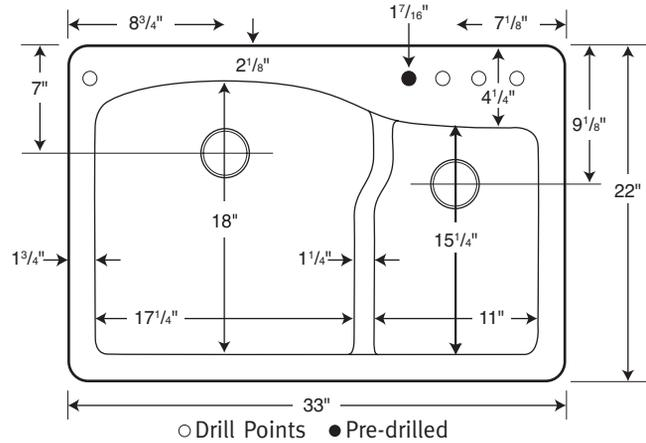
Capacity: 8-1/2 gallons in large (left) bowl until it reaches the divider height, 2-1/4 gallons in small (right) bowl until it reaches the divider height
