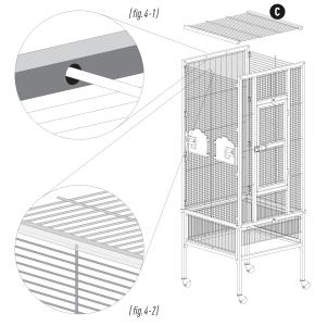
When all extended wires and corresponding holes are aligned, secure the **center top** [C] panel with a long hex screw in each corner.
